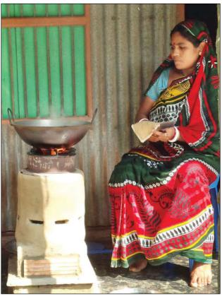
He explained how it works: "The stove produces a different type of byproduct which can easily be used as a fertiliser because of the burning process of the stove. This is how it only burns the gas of the biomass but not all the matter."
